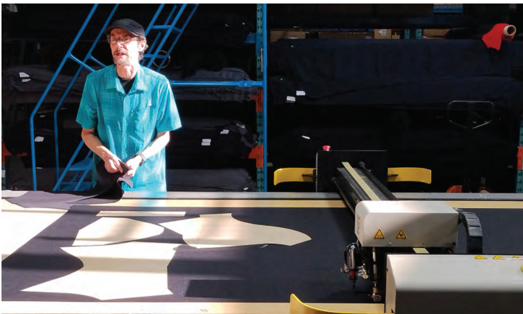
Vacuum cutting table on which a suit can be cut in three minutes.
