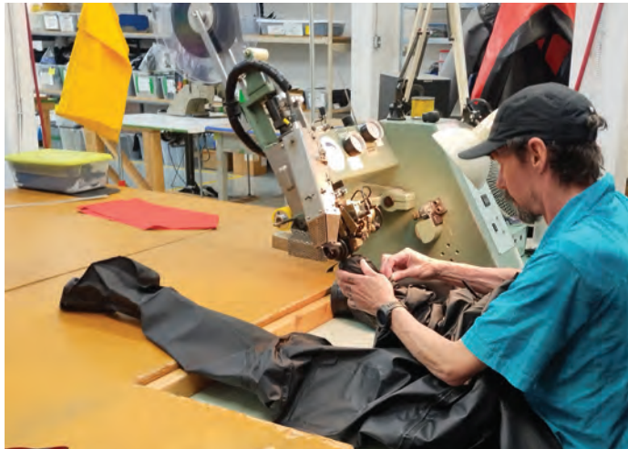
Welding the seams of a suit using a 600 degree welder.
